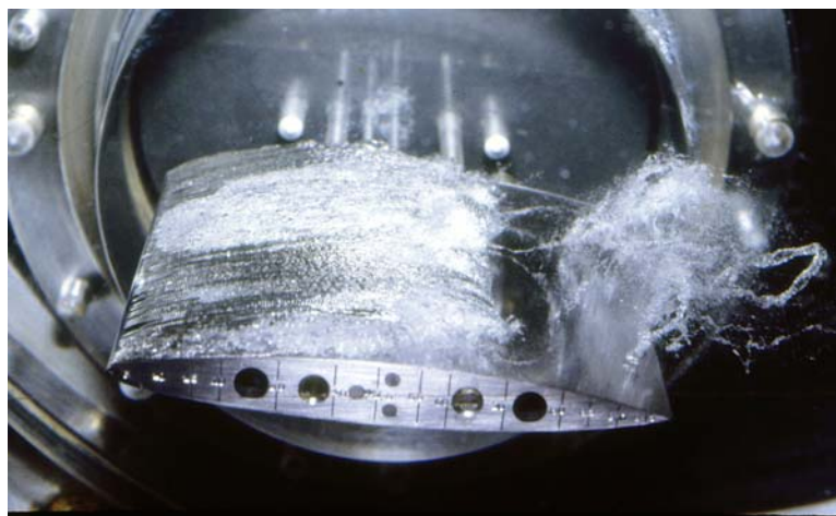
Figure 30: The Cloud Cavitation Instability and the Shedding of a Cloud by a Partial Cavity.
