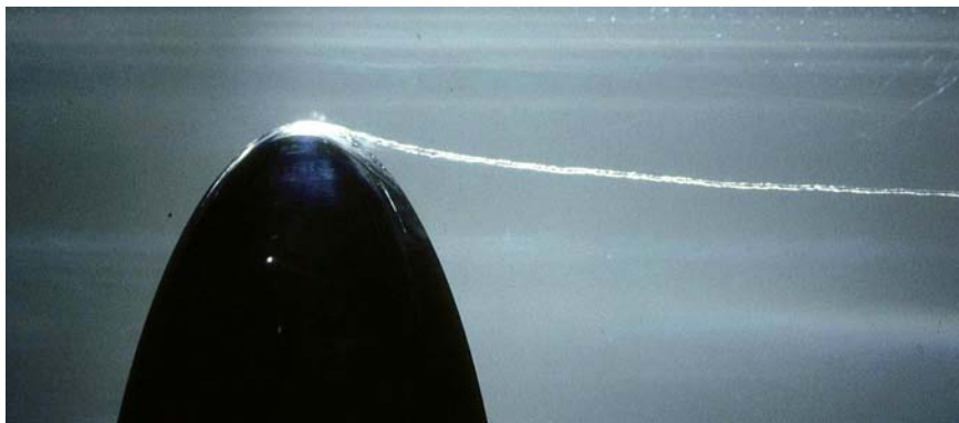
Figure 6: Vortex Cavitation Generated by a Three-Dimensional Hydrofoil.
